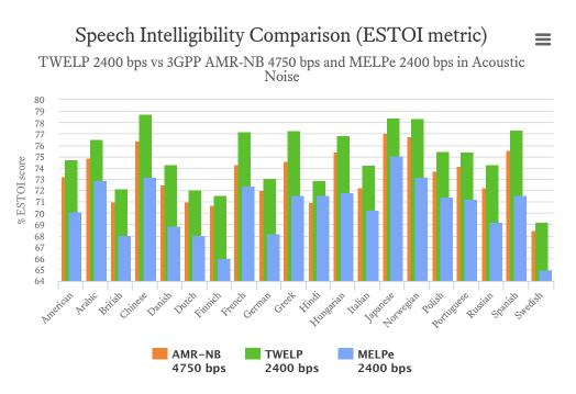
The diagram demonstrates the advantage of the TWELP 2400 bps vocoder over both the MELPe 2400 bps and AMR-NB 4750 bps vocoders, despite the latter operating at twice the bitrate. Exact numbers are shown in the table below.
