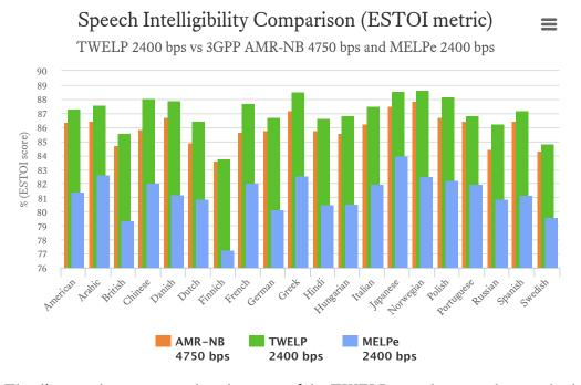
The diagram demonstrates the advantage of the TWELP 2400 bps vocoder over both the MELPe 2400
