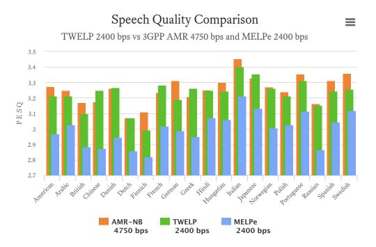
The diagram demonstrates that the speech quality of the TWELP 2400 bps vocoder is closer to that of the AMR-NB 4750 bps vocoder and significantly better than that of the MELPe 2400 bps vocoder. Exact numbers are shown in the table below.
