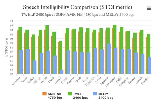
The diagram demonstrates the advantage of the TWELP 2400 bps vocoder over both the MELPe 2400 bps and AMR-NB 4750 bps vocoders, despite the latter operating at twice the bitrate. Exact values are provided in the table below:
